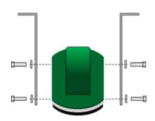
3. Once the cable is installed, attach the right and left angle brackets to the to the cable head using the four  $\frac{1}{4}$ " x  $\frac{3}{4}$ " grade 8 bolts and  $\frac{1}{4}$ " flat washers.
