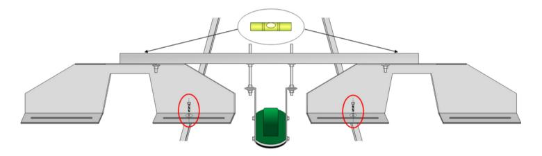
8. Tighten all the screws securing the roof brackets to the ribs of the bin. Tighten the bolts securing the C-channel to the roof brackets. Use the 3/8" nuts installed on the threaded rods to adjust the gap between the C-channel and the angle brackets so that the cable head is appropriately supported.
