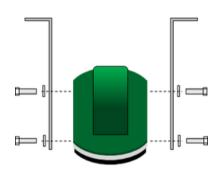
3. Once the cable is installed, attach the right and left angle brackets to the to the cable head using the four  $\frac{1}{4}$ " x  $\frac{3}{4}$ " grade 8 bolts and  $\frac{1}{4}$ " flat washers.
