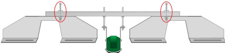
6. Use two  $\frac{1}{4}$ " self-tapping screws and 5/16" fender washers to loosely secure the roof brackets to the two ribs closest to the sensing cable. Attach both self-tapping screws at the same height up the rib so that the C-channel sits level across its length.
