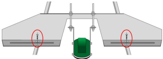
6. Using the 3/8" nuts installed on the threaded rods, adjust the gap between the roof bracket and angle brackets to support the cable head appropriately.
