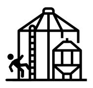
CAUTION Extreme care and caution must be used when climbing up a bin. Be sure to use approved safety procedures and materials such as ladders and a safety harness. When working above 1.2 metres, wear a safety harness or personal protective equipment. An approved tool belt must be worn to keep both hands free when climbing up and down a ladder.
